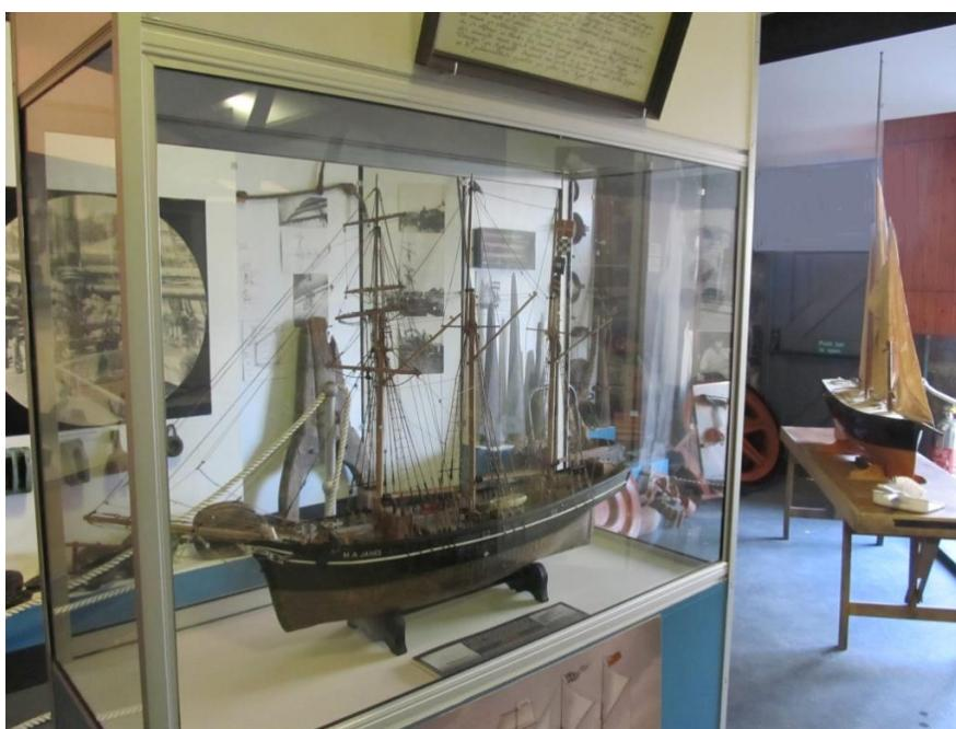
The large model of the "M A James" can be used to show the different parts of a typical "Western Ocean Yacht" – the galley on deck/where the sailors lived etc.
